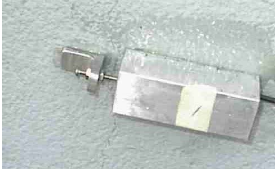
Figure 2.6 LVDT displacement measurement sensor
