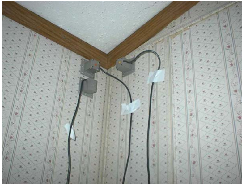
Figure 2.3 Upper corner velocity transducers connected to the S2 seismograph
